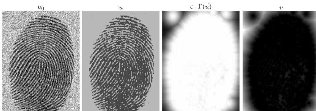
FIGURE 12. The segmented fingerprint using the Ambrosio-Tortorelli approximation with  $\lambda = 1000$ ,  $\varepsilon = 15$
