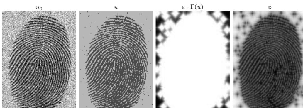
FIGURE 13. The segmented fingerprint using the infinite laplacian approximation with  $\lambda = 20$ ,  $\varepsilon = 15$
