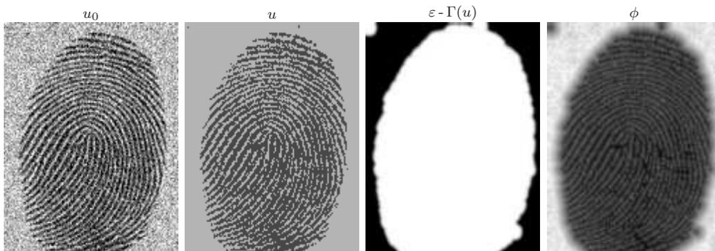
FIGURE 6. The segmented fingerprint using our presented model, approximated through the Lipschitz level set method, with  $\lambda = 20$ ,  $\varepsilon = 40$ .
